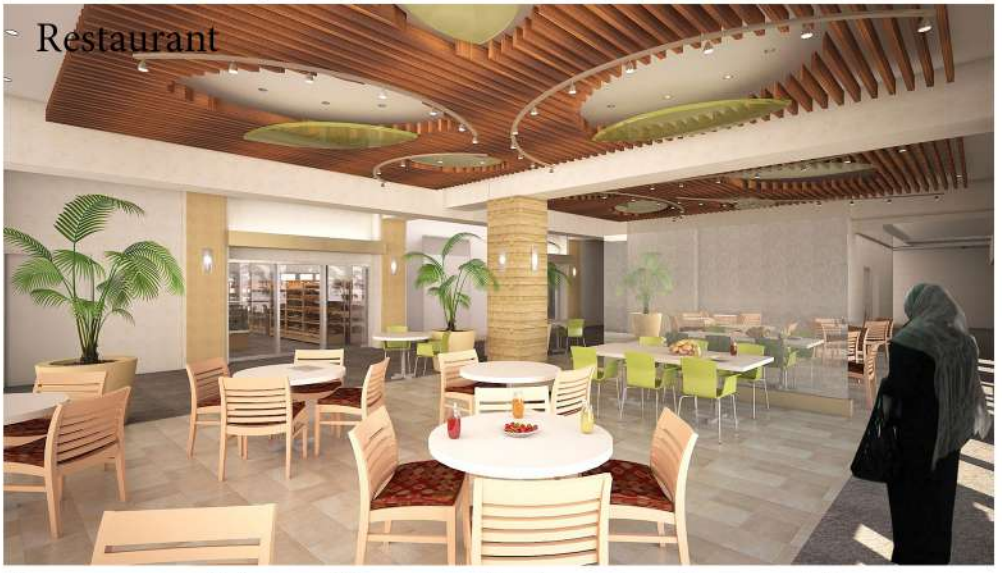
Restaurant false ceiling are designed using wooden battens by providing the cut outs in the form of leaf .
